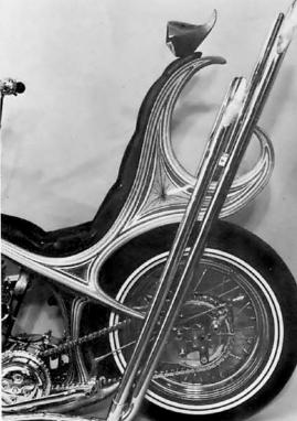
show the extensive chrome plating done by South Shore Plating Company, Quincy, Mass. Besides undergoing the flawless filling and molding treatment, the frame was raked a full 3 inches at the steering head and fitted with a circa 1930's Velocette girder fork. The auxiliary side springs were removed for a cleaner appearance. Believe it or not, the ancient fork and steering races fit the Triumph neck with no modifications. (Everyone
