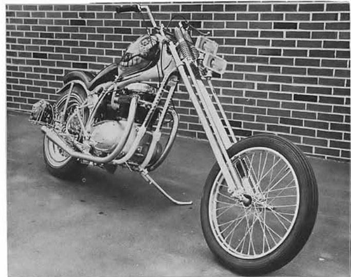
Stock Beezer head pipes complete with balancing tube run into a set of custom upsweep mufflers.
