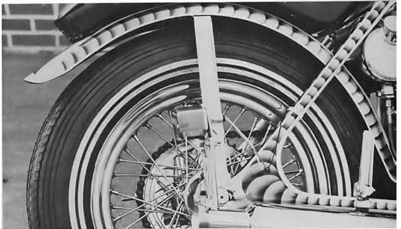
Hefty fender brace made by Martin supports a flat fender from Cheat'ah.
